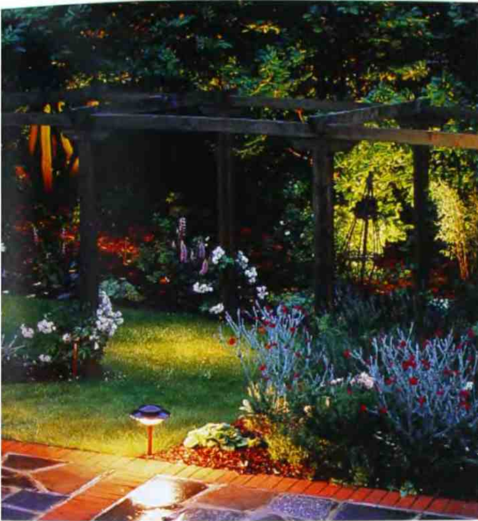
left: Regularly spaced spreadlights provide effective pathlighting without detracting from other illuminated garden features along the route.
