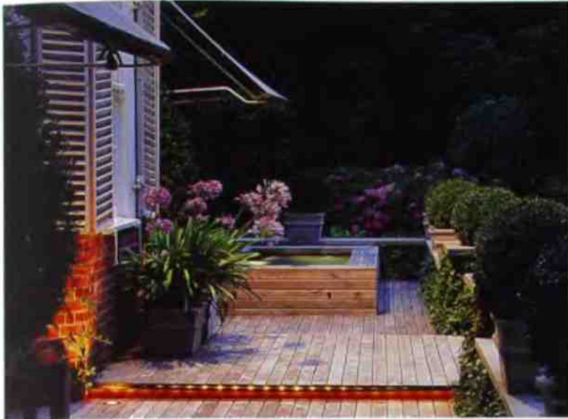
left: Uplighting of the house façade coupled with downlighting of the decking and linear lighting of the steps produces an impression which is both ornamental and practical.
