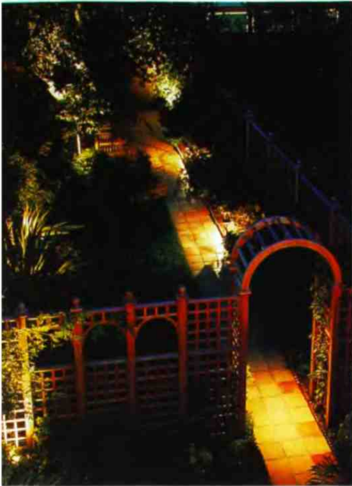
above: A downlight on the arch and spreadlights in adjacent borders provide effective pathlighting. Uplighting of planting provides a sense of space and security along the route.
