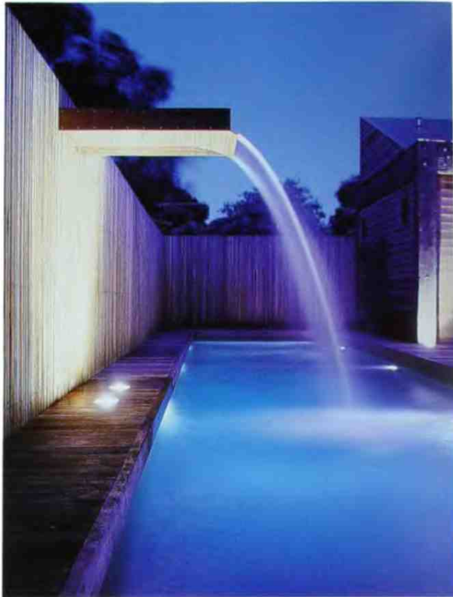
right: Uplighting the plank walls and timber structures provides an architectural framework for recessed crosslighting of this azure lagoon. The sheet of falling water receives light from the luminaires recessed into the decking, as well as from under-water lighting in front.
